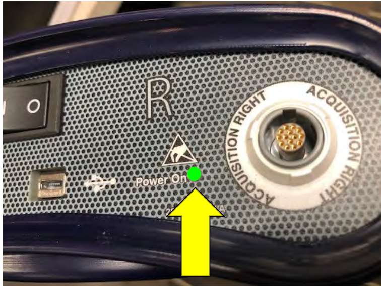
Figure 4: Connection and power up of Head Unit
