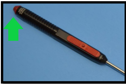
Intact end cap (ok to use)
