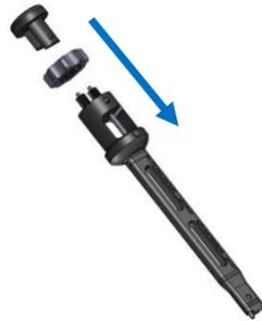
c) Place the Depth Stop Assembly through the Guide and thread it into the Depth Stop Knob.
