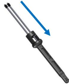
b) Slide the geared ring and impactor cap into body. Secure with thumbscrew (not shown).
