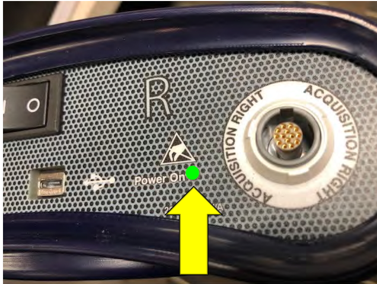
Figure 4: Connection and power up of Head Unit
