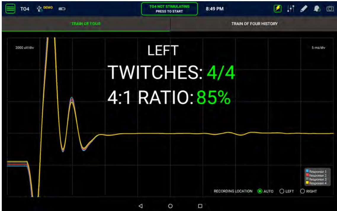
Figure 17: Train of Four showing waveforms
