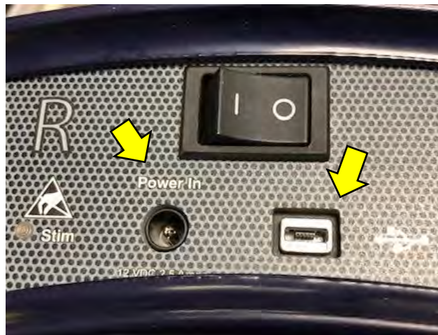
Figure 3: USB and power ports on Head Unit
